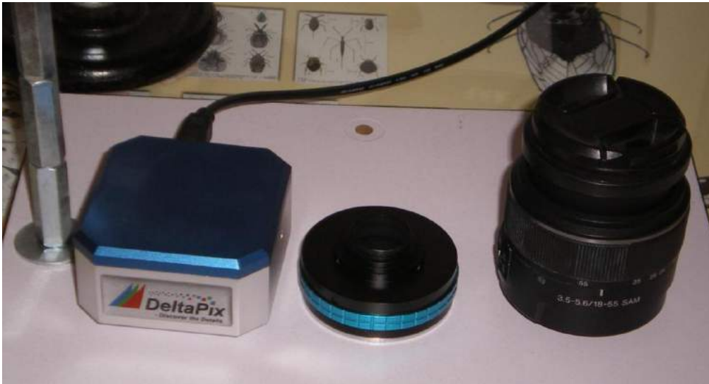
Figure 1. From left to right: DeltaPix Invenio 8DII Camera, C-thread adapter, Sony SAL-1855 lens
