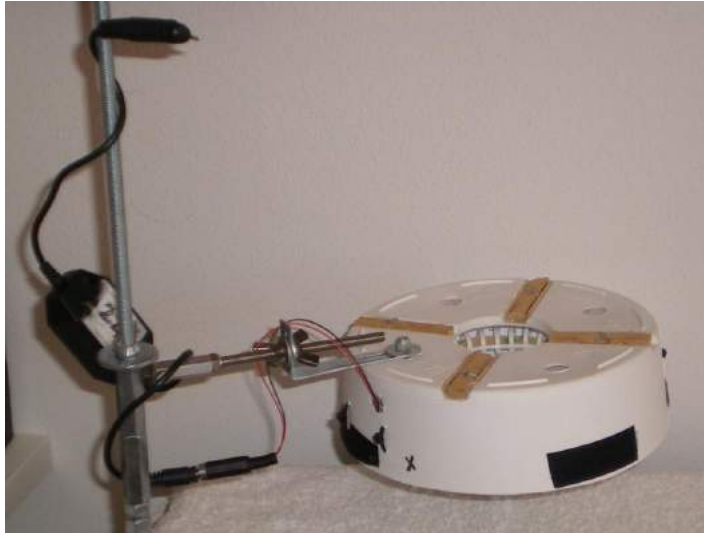
Figure 2. Self-built, diffused light illuminator
