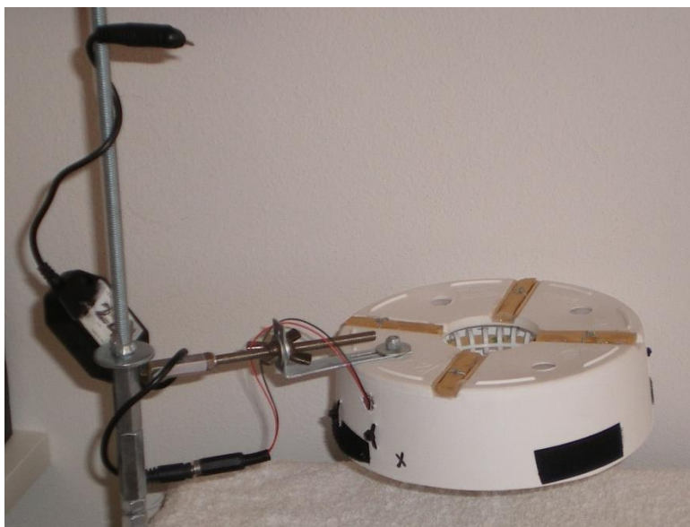
Figure 2 – Self-built, diffused light illuminator
